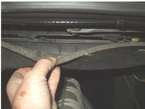
Slide the filter housing to the right. There are three compression sliders on each side of the housing.
