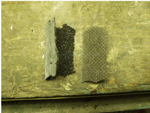
The filter is quite heavy, as it is has carbon sandwiched between the layers. The carbon helps deodorize smells from the outside:
