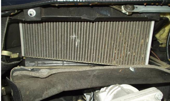
The housing will drop, exposing the filter. Remove the filter and clean out the housing. In my case I had feathers from a bird that hit the hood of the van.
