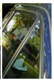
There are two other areas that can be filled with gasket material. First, there is the leading edge of the door around the fender area. This uses gasket style D, with the trailing edge of the gasket cut off for fit and flat-surface gluing purposes.
