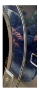
The second area is the trailing edge of the door (area 4 in the picture above). This uses gasket style B. This gasket was also the most difficult to install. Note that on my van I applied this gasket a little too far out, thus causing the contact glue to be visible.
