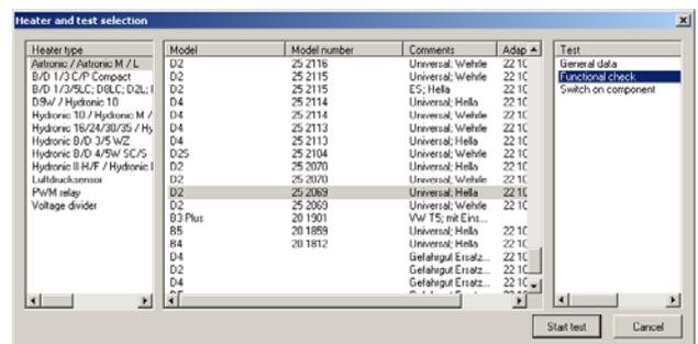
In our example of the Airtronic D2 model 25 2069) there are three possible tests which may be performed; General data, functional test or switch on component.
