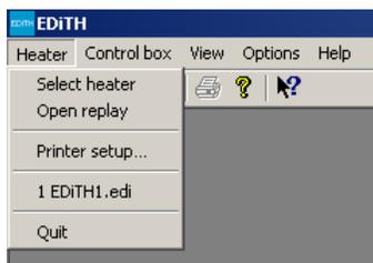
Once EDiTH has been opened and the basic setup has been completed, a heater model must be selected. In the top left corner of the screen is a drop down menu called 'heater', hover the mouse pointer over it and click on 'select heater'.
