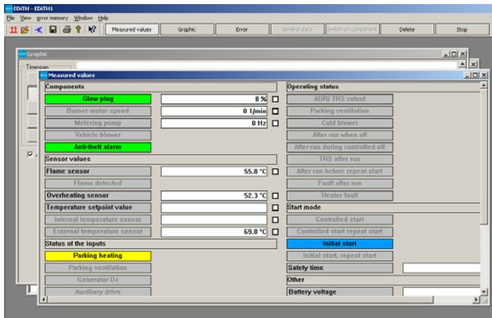
There are two main screen that are of concern; the Measured Values screen and the Graphic screen.
