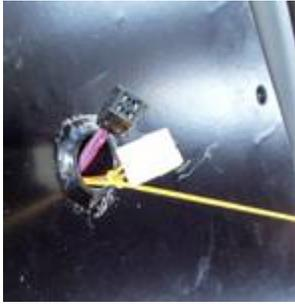
The problem here is the pedestal side of the seat belt line is short, putting the connector into the middle of the conduit. Feed the
