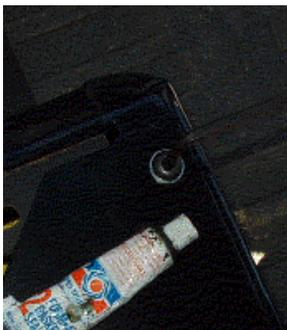
4. Passenger side: Feed the heating electrical through the swivel post. The swivel base has four holes drilled to accept bolts into the pedestal. Use the bolts and washers provided in the packaging to mount the swivel base. Two of the 6 holes in the pedestal are not used. I used Form a Gasket to reduce the chance of vibrational loosening. **Hint:** The holes in the swivel base are slightly tight relative to the base holes. Loosely set all
