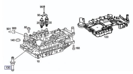
Looking at Mercedes-Benz EPC will give you an idea of components inside the transmission. Here, we have highlighted the oil guide pipe. It supplies fluid pressure to Brake B3. If there is a leak here, it can cause problems with starting — Neutral, 1st and Reverse all need B3.
