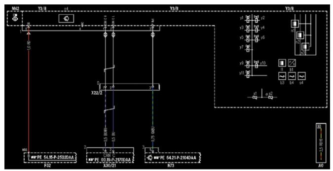
With a paid subscription to www.startekinfo.com, you can view a wiring diagram for the ETC unit. Here we have the 724.2 showing the power supply, CAN C, and wake-up signal. The transmission body itself forms the ground for all the electrical components.
