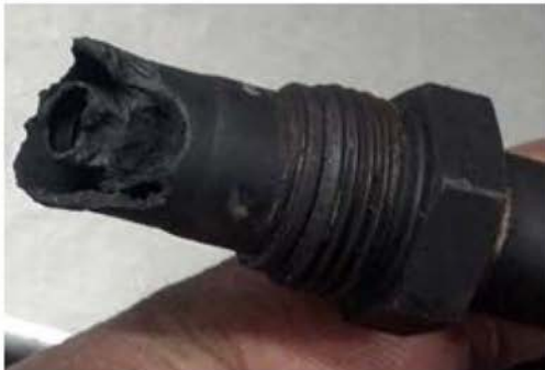
Melted NOx Sensor
