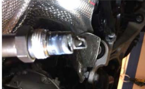
Melted NOx Sensor
