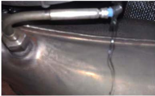
Melted Temperature Sensor Insulation (before DPF)
