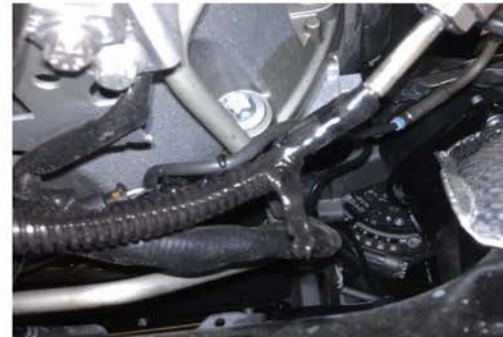
Melted Temperature Sensor Insulation (near Turbo)
