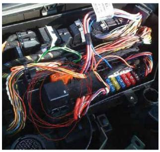
These days pulling fuses one at a time while watching the milliamp draw reading taken between the negative battery post and the cable clamp is "Verboten." Instead, read the mV drop across the fuse, then convert that to mA.
