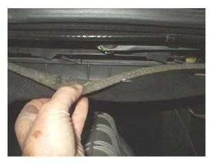
Slide the filter housing to the right. There are three compression sliders on each side of the housing.
