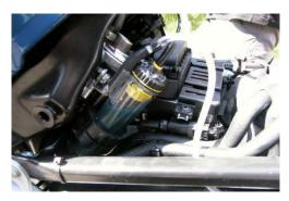
The delivery tubing can be routed along the swingarm using conduit and glue or self adhesive cable clips and the dispenser can be secured on the rear spindle using a Dispenser plate & Clip. For further information see our easy step installation guide - <u>Dispenser Assemblies</u>, <u>General</u>. The nib should feed the rear sprocket between the 6 & 7 o'clock positions, with the cut face outwards.
