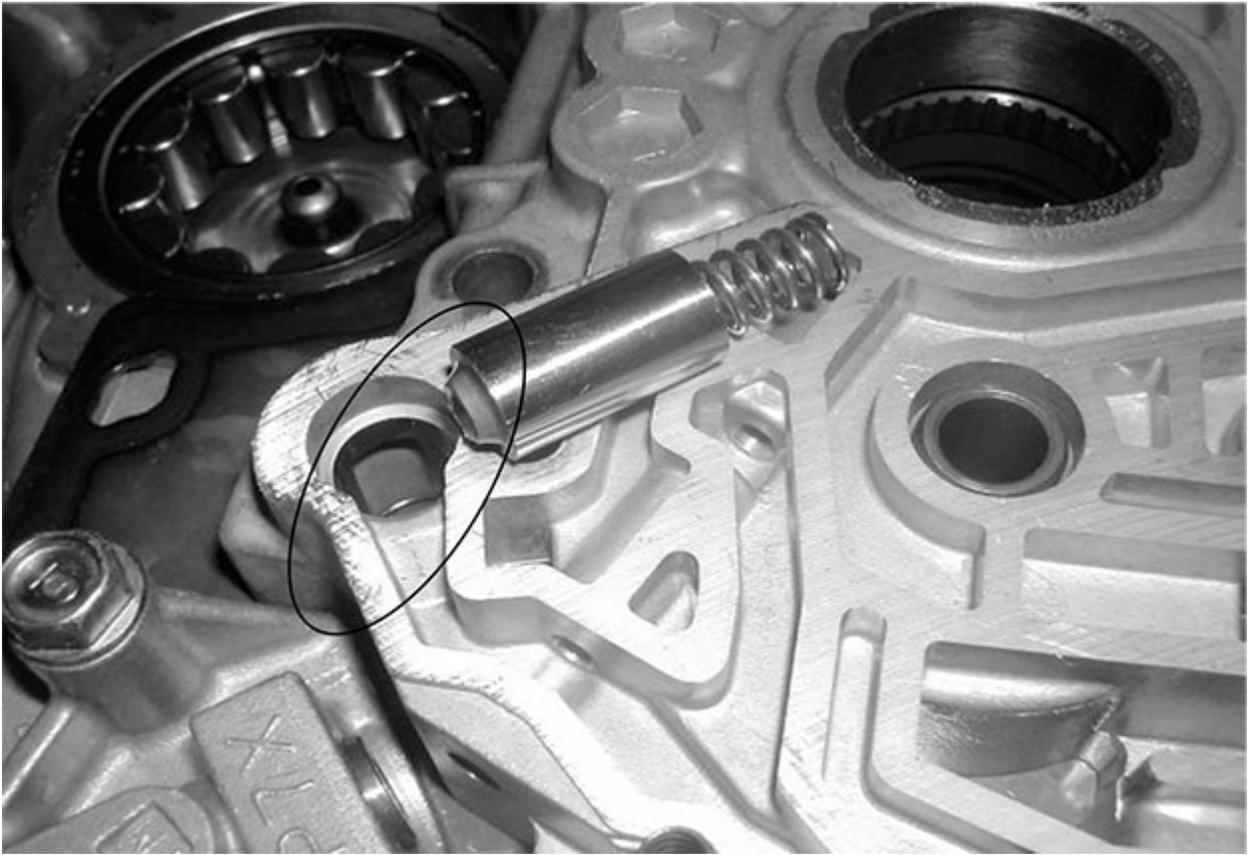
Loss of TCC or TCC slip: Created by end plug loose at the TCC control valve. A cross leak of converter charge oil into TCC control negatively affects TCC control. Inspect the stator for cross leakage at the finished area, where it passes through the casting.
